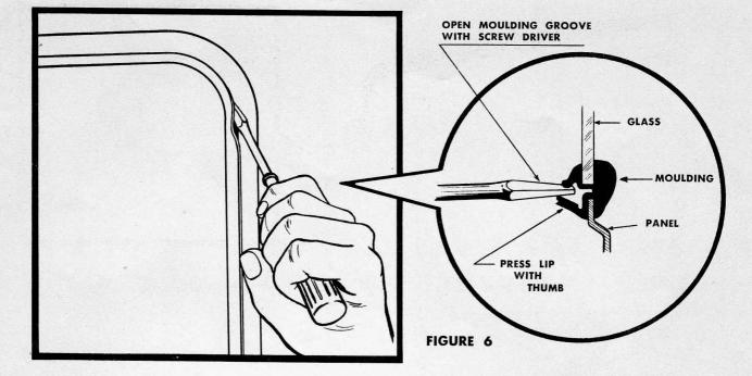
The final operation is to lock the rubber moulding. Insert a small screw driver in opening of moulding as shown in Fig. 6 and the pop-up. Then, by moving the tool along the opening, and following with thumb pressure, the molding lip locks into position securely.
